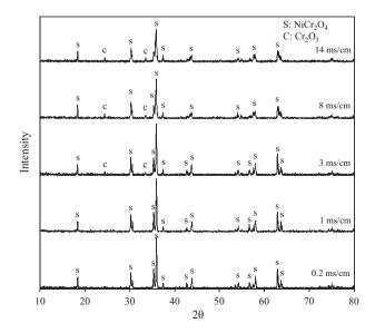
Fig. 4. XRD patterns of samples (with a Cr/Ni ratio of 2) with different conductivities sintered at  $1200 \,^{\circ}$ C.
