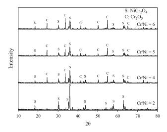
Fig. 7. XRD patterns of samples (with a conductivity of 3 ms/cm) with different molar ratios sintered at  $1200 \,^\circ$ C.
