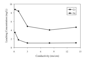
Fig. 6. Leaching concentrations of samples (with a Cr/Ni ratio of 2) with different conductivities sintered at 1200  $^\circ$ C.
