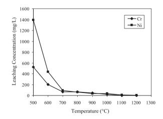
**Fig. 3.** Leaching concentrations of samples (with a Cr/Ni ratio of 2 and a conductivity of 1.4 ms/cm) sintered at different temperatures.
