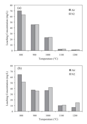
**Fig. 10.** Leaching concentrations of samples (with a Cr/Ni ratio of 2 and a conductivity of 0.2 ms/cm) sintered at different temperatures under two atmospheres.
