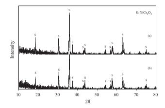
**Fig. 9.** XRD patterns of samples (with a Cr/Ni ratio of 2 and a conductivity of 0.2 ms/cm) sintered at  $1200 \degree$ C under two atmospheres of (a) N<sub>2</sub> and (b) air.
