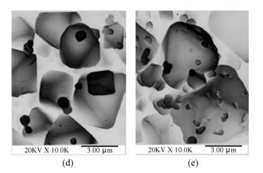
Fig. 5. SEM micrographs of samples (with a Cr/Ni ratio of 2) with different conductivities of (a) 0.2, (b) 1, (c) 3, (d) 8, and (e) 14 ms/cm.
