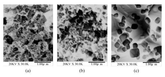
Fig. 2. SEM micrographs of samples (with a Cr/Ni ratio of 2 and a conductivity of 1.4 ms/cm) sintered at (a) 500, (b) 800, and (c) 1200 °C.
