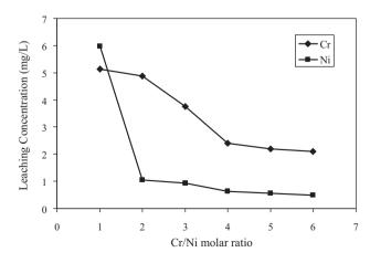
Fig. 8. Leaching concentrations of samples (with a conductivity of 3 ms/cm) with different molar ratios sintered at  $1200 \,^{\circ}$ C.
